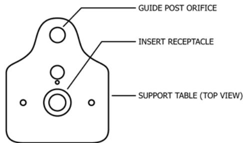
TYPICAL TABLE INSERTS USED FOR POSITIONING TUBING, O-RINGS AND SMALL SPECIMENS
