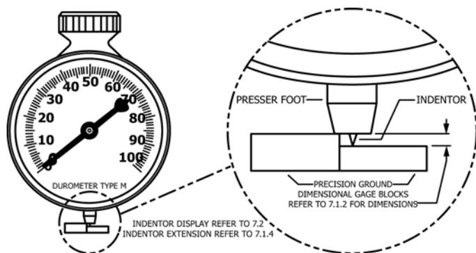
FIG. 4 Detail of Indentor Extension and Display Adjustment
